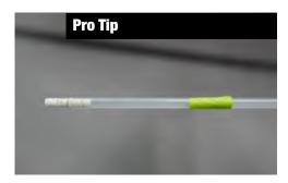
Mark the end of the Rigid 360° Applicator with masking tape to keep from spraying outside the panel.
