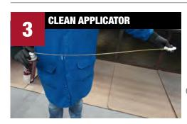
Clean Rigid 360° Applicator by attaching the tip and Applicator to XXX Universal Gun Cleaner.
